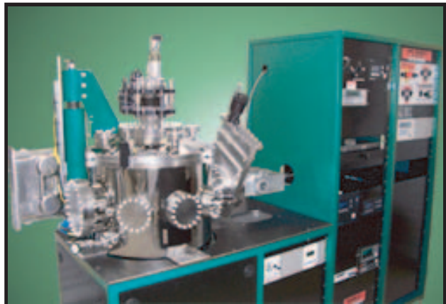
ATC 2200 IBAD with (3) A340-XP 4" UHV sputter sources with in-situ tilt, a COPRA ICP plasma/ion source for ion beam assisted deposition below 5 \times 10^{-4} Torr, 1200 l/s turbopump, 800°C rotating substrate heater with RF bias, computer control and a load-lock for 6" diameter substrates.
