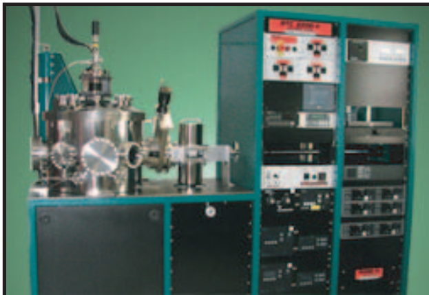
ATC 2000 with (6) A320-XP 2" UHV sputter sources with in-situ tilt, 1200 l/s turbopump, 850°C rotating substrate heater with RF bias, computer control and (6) substrate cassette elevator in the load-lock for 4" substrates.
